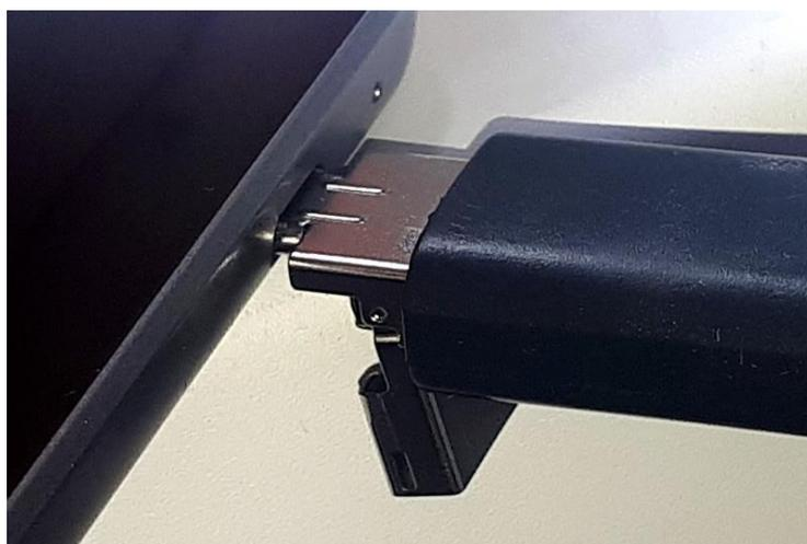
**Figure-19: The USB port of the display (option) is situated on the lower edge of the device. Mind the correct position of the connection**
