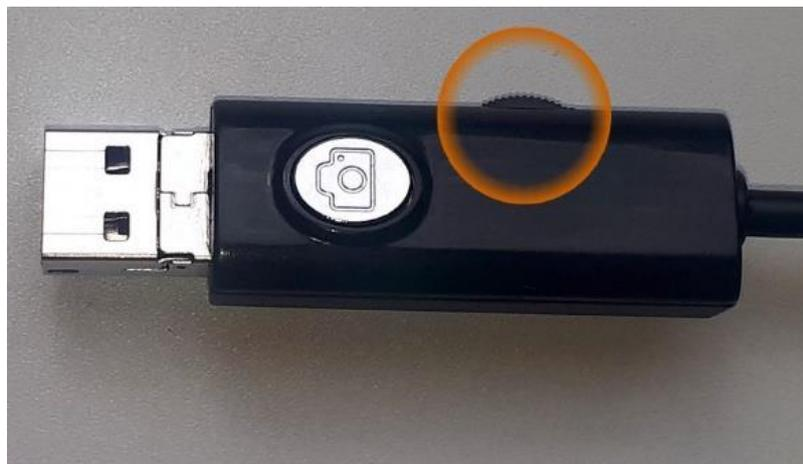
Figure-20: The power of LED lights can be adjusted with the knob (framed)
