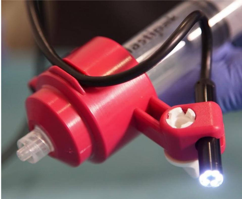
**Figure-11: Mounting the camera. The body of the camera is placed in the small slot to the right. The screw (below the camera, white) is used for fixing the position of the camera. The cable can be pushed into the channel (left), which makes the way free for the syringe (in the background)**
